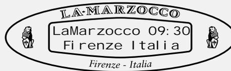
The digital display (display) is a backlit display capable of displaying 2 lines of 16 characters. The display enables the operator to interact with the espresso machine to visibly change parameter values. The display also provides valuable information to the operator.
